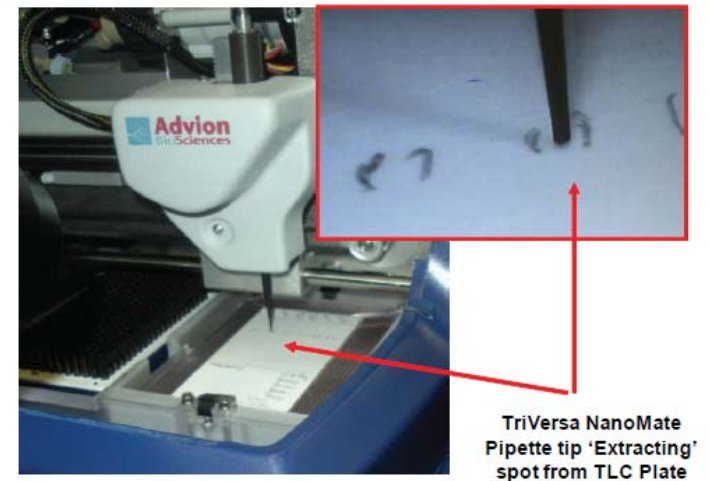
Figure 1 LESA-Enabled TriVersa NanoMate for Surface Sampling
